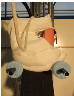
Figure 8. The Hövding2.0 and the larger anvil
