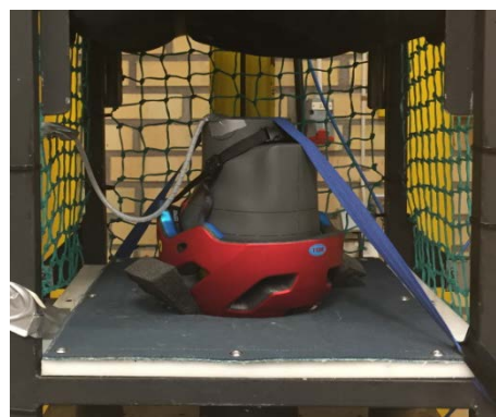
Figure 2. The method used in shock absorption test
