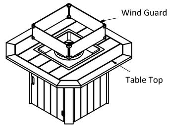
8. See Wind Guard Assembly Instructions and assemble. Place on Firepit Table Top.
