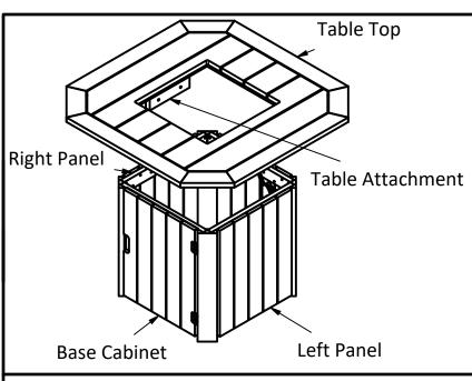
1. Align the Table Top so that it sets into the Base Cabinet. The Top will have (2) Table Attachment pieces with (2) holes in them. This is what attaches the Table Top to the Base Cabinet.
