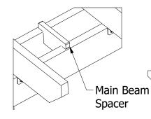
**24)** Place the Main Beam Spacer Between the Lower Support Beams as Shown Above to Maintain the Correct Beam Spacing.
