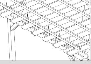
**32)** Secure Each Remaining Top Slat with (7) "D" Screws.
