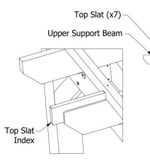
**29)** Use the Top Slat Index to Set the Location of the First Top Slat. Set the Top Slat Index on Top of the Joist as Shown Above, and Adust the Top Slat Until it Rests Against the Top Slat Index.
