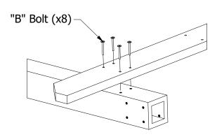
**6)** Attach the Lower Support Beam to Each Post Using (4) "B" Bolts.
