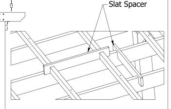
**31)** To Set the Location of Each Subsequent Top Slat, Use the Slat Spacer to Set the Center-to-Center Distance Between Top Slats. Use the Second Slat Spacer to Maintain Proper Spacing of the Joists as Shown Above. Move Each of the Spacers Accordingly so they are Near the Area of the Top Slat Being Secured. This will Ensure all Slats Remain Straight and Square with One Another.
