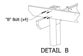
**13)** Lift an Upper Support Beam into Place as Shown and Set on Top of the Lower Support Beams. Secure Both Ends to the Posts Using (8) "B" Bolts, as Shown in Details "A" and "B".
