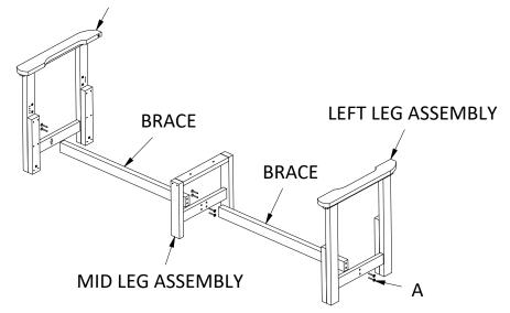
1) Attach Braces to Leg Assemblies using (8) A Bolts.
