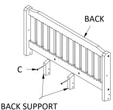
**3)** Attach Back Supports to Back using (1) C Bolt for each Back Support as shown.
