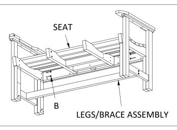
**2)** Attach Seat to Legs/Brace Assembly using (4) B Bolts as shown.
