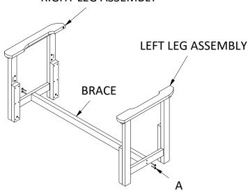
1) Attach Brace to Leg Assemblies using (2) A Bolts on each side.
