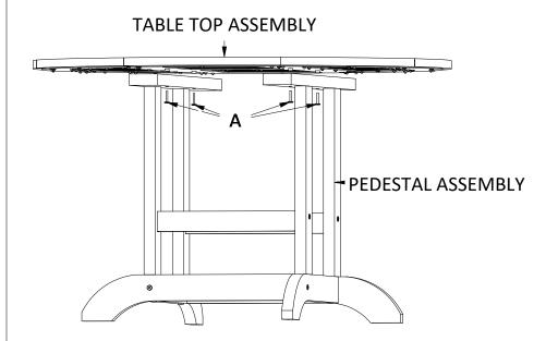
5) Place the Table Top Assembly on the Pedestal Assembly and attach together using (4) A Bolts.
