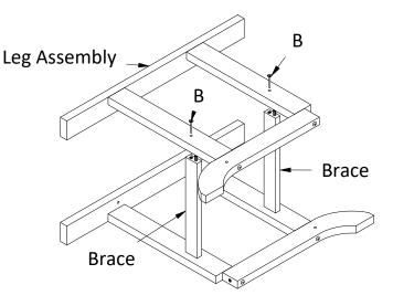
2) Attach the Leg Assembly to the (2) Braces with (2) B Bolts.
