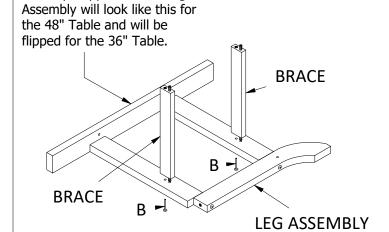
1) Attach the (2) Braces to the Leg Assembly with (2) B Bolts.
