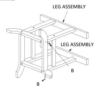
4) Attach the Foot to both of the Leg Assemblies with (2) B Bolts.
