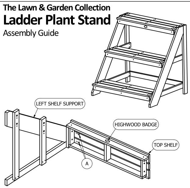
**1)** Place Left Shelf Support on Flat Surface as Shown. Slide Top Shelf (With Elk Outdoor Badge) Over Top Support and Attach Using Two "A" Bolts.
