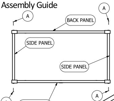
1) Place Front Panel on Flat Surface With Inside of Panel Facing Up. Insert the Dowels in the Side Panels into the Holes on the Front Panel and Fasten with (4) "A" Bolts Thru Holes in Legs. Repeat for the Back Panel.
