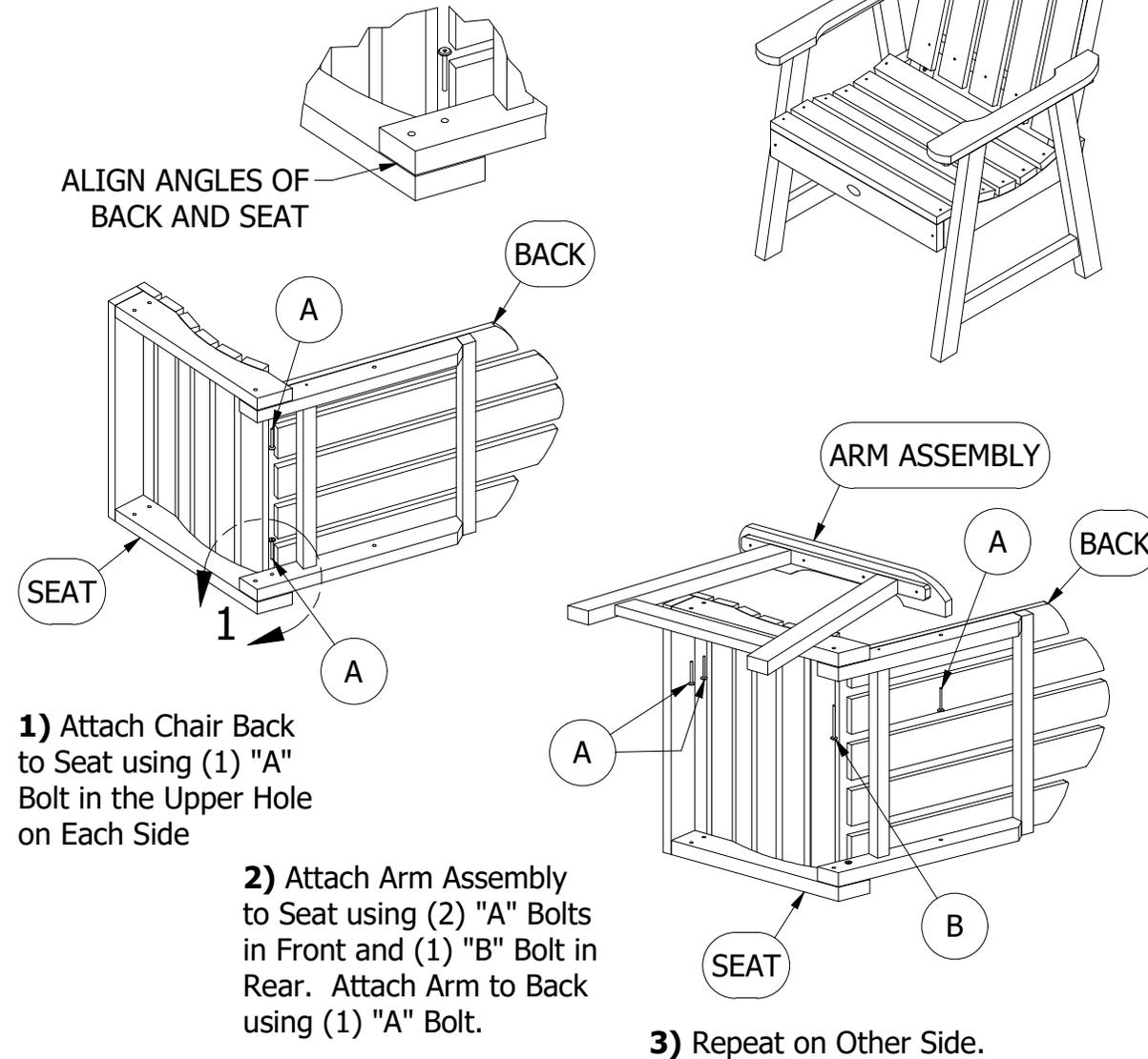
**1)** Attach Chair Back to Seat using (1) "A" Bolt in the Upper Hole on Each Side
