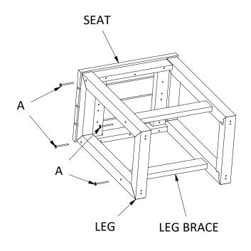
1.) Place the Seat onto its side and attach the Leg & Leg Braces with (4) A Bolts as shown. Repeat this step on the other side.
