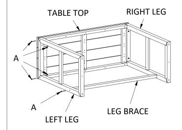
1.) Place the Table Top onto its side and attach Either the Left or Right Leg and Leg Brace using (5) A bolts As shown. REPEAT THIS STEP ON THE OTHER SIDE
