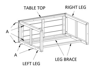
1.) Place the Table Top onto its side and attach Either the Left or Right Leg and both Leg Braces using (6) A bolts As shown. REPEAT THIS STEP ON THE OTHER SIDE
