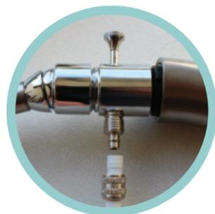
5. Connect the FLO's tubing to the diverter seating it fully over the stem. Then tighten the compression nut.
