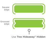
Use Trex Hideaway® Hidden Fastening System for a clean, fastener-free appearance
