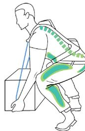
Diagram of proper lifting posture with ErgoSkeleton™
