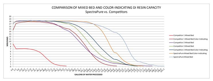
Since pure water is a poor conductor of electricity, purity is best measured using resistivity (megohms) or its inverse, conductivity (microsiemens). Water is considered to be ultrapure when the resistivity is 18.2 megohms. This is represented by the vertical axis on the above chart. The horizontal axis represents the total number of gallons processed.
