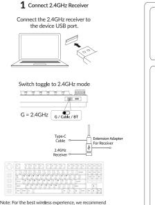
Note: For the best wireless experience, we recommend using the extension adapter for receiver and putting the 2.4GHz receiver somewhere on your desk close to your keyboard for a low rate of latency and fewer signal interferences.
