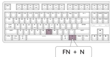
6-key rollover: the keyboard can detect up to 6 simultaneous key inputs.
