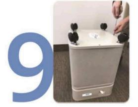
Replace the bottom cover & screw down tightly
