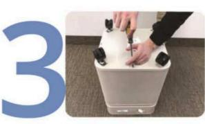
Using a Phillips screwdriver, remove the four retaining screws from the bottom cover
