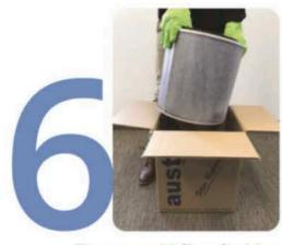
Remove old filter & old prefilter from unit & place into empty box
