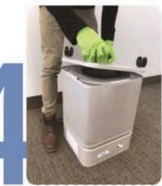
Wearing a protective pair of gloves, lift the bottom cover off & set aside
