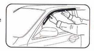
Once you are satisfied with the alignment, carefully peel off a small part of the tape backing from each corner of the deflector leaving the plastic tab exposed. Stick the corners of the wind deflector to your vehicle and then peel off the rest of the adhesive backing using the exposed tabs.
