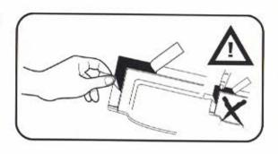
Now your Wind Deflectors are installed and all the adhesive backing has been removed, apply firm pressure along where the tape is located to ensure a good bond between the Wind Deflector and the door frame.
