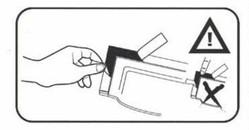
Once you are satisfied with the alignment, carefully peel off the backing from the tape and install....
