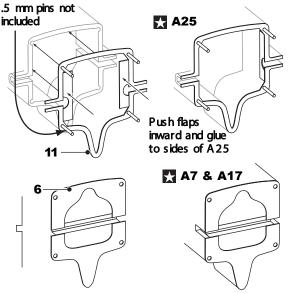
Bend part #6 to the shape shown (Profile). Mount onto parts A7 and A17 to form the bulkhead.
