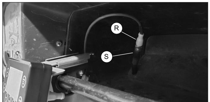
15. Adjust angle of display as best suited for operation and tighten p-clamp to grab bar.
