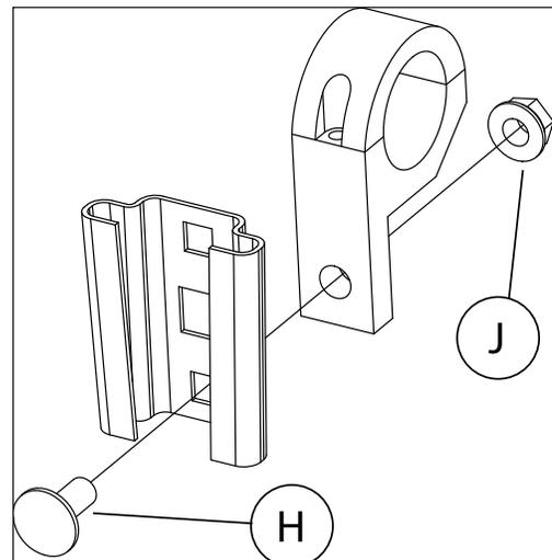
11. Attach the p-clamp to the left side of grab bar in the glove box. Do not fully tighten.
