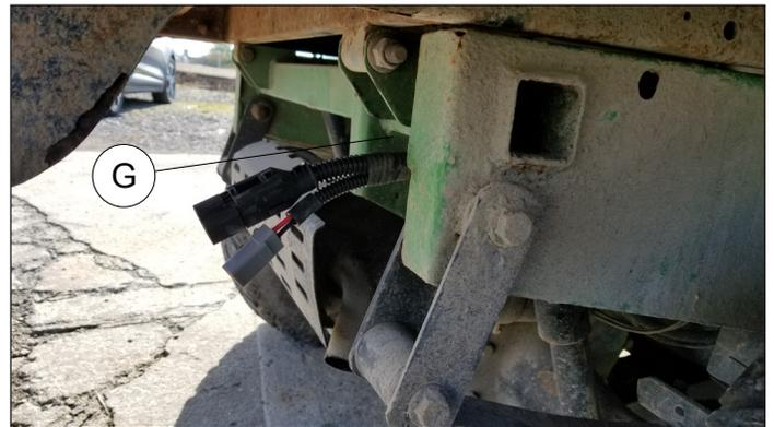
9. Pull slack from both ends of the harness into the battery compartment and secure with a wire tie. Tighten wire tie on inside of frame rail.
