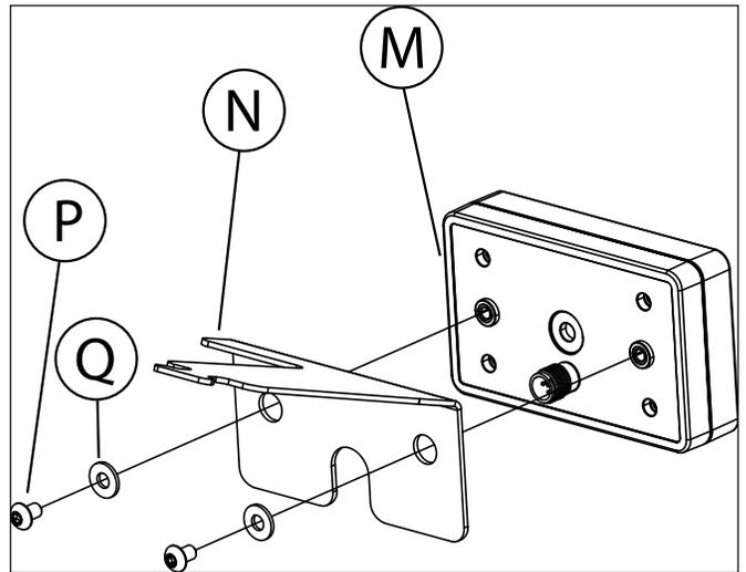
**NOTE:** Tighten the screws to 4-5 ft-lb. Do not over tighten or damage may occur to the threaded inserts and plastic housing.
