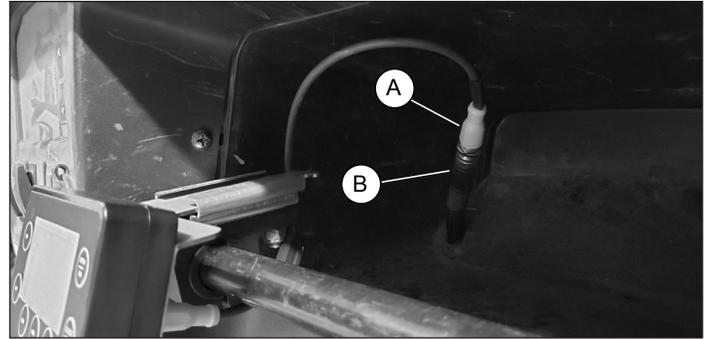
2. Remove display by sliding bracket out of the receiver.
