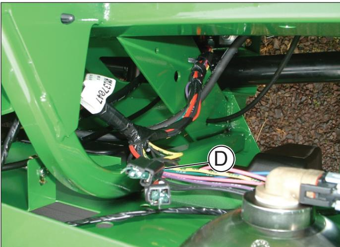
6. Raise the cargo bed and route the other end of the power harness from the battery compartment into the engine compartment on the inside of the right-side frame rail and lightly secure to the vehicle harness with a wire tie.
