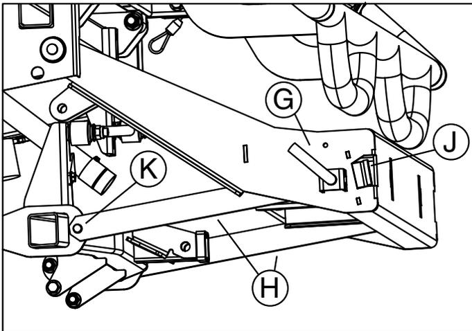
3. Release side pins (G) and lift frame until it clicks into place. Be sure the frame is locked in position before mounting attachment.
