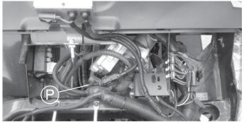
8. Bring the 12 foot extension end (P) up and plug into the control box. Tie the end to the larger conduit in a place where it can be conviently plugged together and pulled apart.
