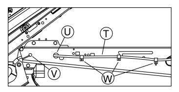
11. From the battery compartment route the 12 foot extension (T) rearward along the outside of the vehicle frame through the large hole (U) and out the end of the frame tube. Connect the end with the free end on the attachment mounting frame (step 10 part (S)) and pull the wire forward as far as possible. Wire tie the wire to the Gator frame through hole (V). (Leave enough wire sticking out the end of the tube that the connection can be made and pulled apart without too much trouble).
