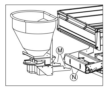
6. Slide receiver arms (M) into the slots (N) until it clicks to lock into place. Be sure the hitch latches securely. Adding grease to the slots makes installation easier. (It is recommended that two people lift the spreader into place)
