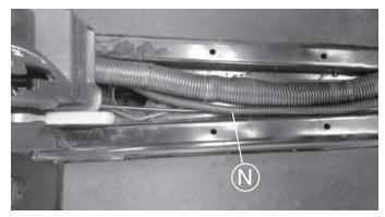
7. Route the 12 foot extension wire (N) from the battery compartment down into the center channel and bring it all the way forward along side the existing larger conduit.
