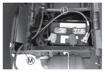
6. Lift the passenger seat to access the battery compartment. Route the male end of the 12 foot extension (L) into the battery compartment through the gap behind the seat (M).
