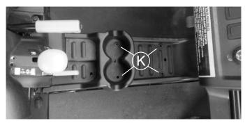
5. Pull the four plastic pins (K) to remove the center console cover.
