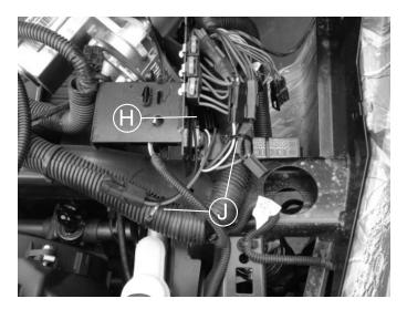
4. Tuck the relay (H) under the bundle of wires and wire tie (J) both ends of the harness to existing conduit.
