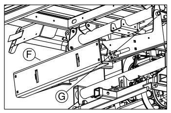
3. Attach Frame Assembly (F) to utility vehicle using two 1/2" x 2" Clevis Pins through holes drilled during step 1 (G). Fasten clevis pins with bowtie clips. (recommend two people do this installation)
