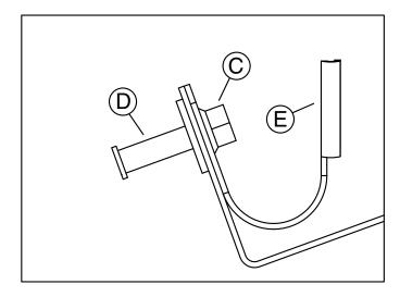
2. Open hood and remove plastic storage tray. Remove the nut (C) from the hood latch pin (D). Attach the Control Box Mounting Bracket (E) to the end of the bolt and replace nut (C). To ensure the hood latches properly, replace bolt in the same position as removed. Mount the control box.
