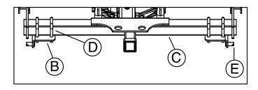
2. Loosely attach the Left and Right Lower Support brackets (B) to the hitch tube (C) as shown using four u-bolts (D) and eight 3/8" flange nuts. Slide the brackets on the tube to line up the end of the pin (E) flush with the outside surface of the plate welded to the hitch tube.
