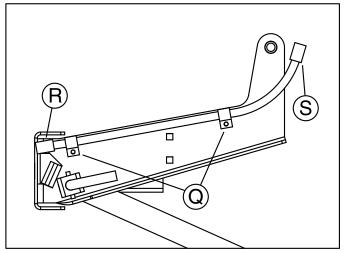
10. Insert two push in cable clamps into the two holes (Q). Plug the female end (R) of the two foot wire extension together with the connector on the spreader. Pull the wire as far forward on the machine as possible and clamp it into place. (Leave enough slack that the connection can be made and pulled apart without too much trouble).
