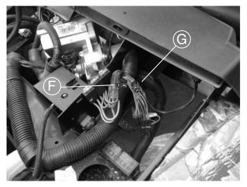
3. Run power wire harness from the control box under the dashboard to behind the steering console. Plug into the two mating plugs (F & G).
