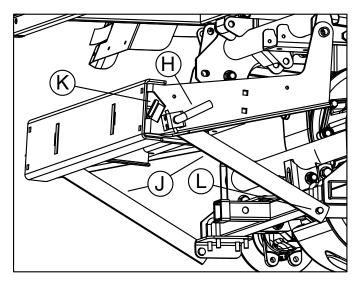
4. With the side pins (H) locked out (pull and turn), slide Supports (J) through the slots in the Frame Assembly at location (K) with the bent end at the top facing towards the outside. Place lower holes over the pins on the Lower Supports (L) and secure with bowtie clips.
