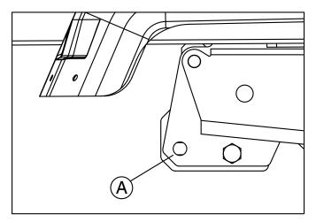
1. At rear of utility vehicle frame, just below where the bed pivots, use 33/64" drill to enlarge hole (A) on both sides of utility vehicle.
