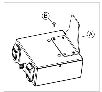
1. Connect Control Box Post (A) to bottom of control box using four #6-32 screws (B) as shown.
