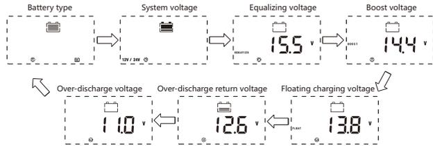
After entering into the setting interface, tap the Set key to switch the menu for setting, and tap the Up or Down key to increase or decrease the parameter value in the menu. Then tap the Return key to exit (without saving parameter setting), or press and hold the Set key to save setting and exit.
