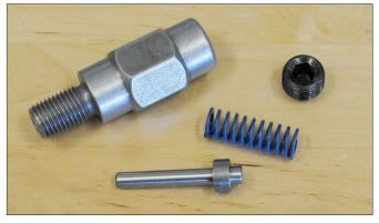
4. You may notice some grey residue around the threads of the set screw. This is conventional plumber's pipe dope that we install on initial assembly to
