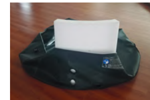
3) Add the foam wall segment with the three holes in it for connection to the base liner.
