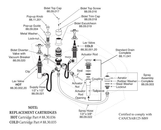
**NOTICE:** These instructions do not represent step-by-step directions. They are a product supplement only to be used by a qualified/licensed plumber. We recommend all plumbing fixtures be installed by a professional.
