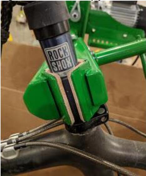
4. Rotate the Clamping Handle clockwise to tighten the clamp. (Be careful not to damage any bike components.) (See Figure 17)
