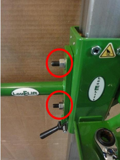
2. Slide the thimble completely over the upper nut. (See Figure 11)
