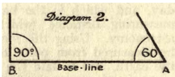
Now if we know the length of the base-line A—B, in feet, yards, kilometres or miles, (to be ascertained by actual measurement), and also know the value of the two angles which indicate the direction of a distant object as seen from A. and B., we can readily complete the triangle and so find the length of its sides. In this way, we can measure the height of a tree or church steeple from the ground level, or find the distance to a ship or lighthouse from the shore.
