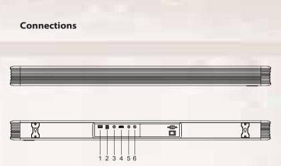
**1. USB IN:** Used to connect a flash drive for direct MP3/WAV playback (FAT32 format and 32GB max).
