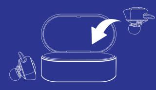
NOTE: To switch to stereo mode, simply take the earbud (L/R) out of the case & place it in your ear. The earbud will automatically power on & pair with each other hence enabling it for stereo usage.
