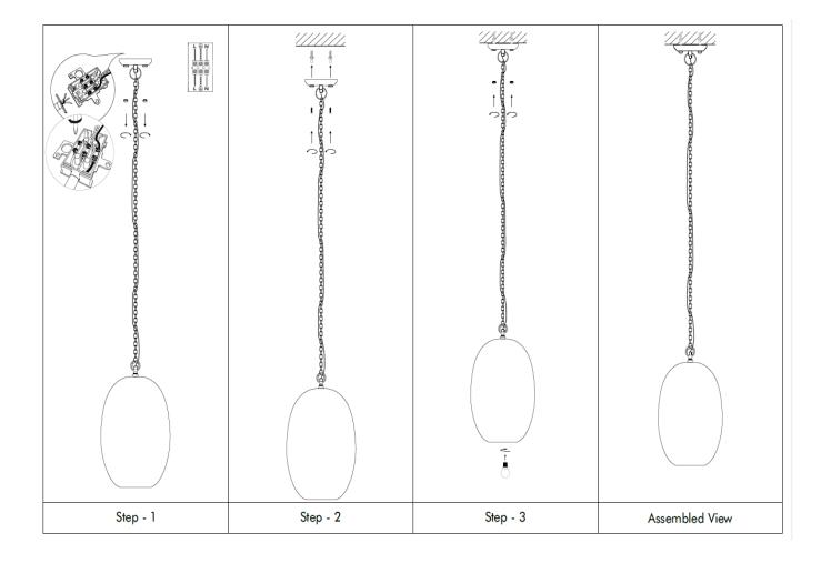
Make sure you have the following items which are required to install this light fitting: Small electrical screwdriver, cross head screwdriver and insulation tape.
