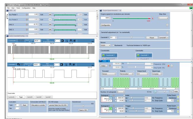
The screenshot shows the MicroLC Software with analog outputs, crank-/ camshaft, RPM and complex PWM.
