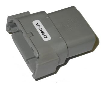
Six versions of Dual Magnetic Converters (DMCs) are available (A, B, C, D, E, F). DMCs convert magnetic style signals to an open collector output signal (square wave). This makes a typical magnetic sensor behave as a switched or hall effect sensor, thus making the signals suitable for use with ECUs and loggers.
