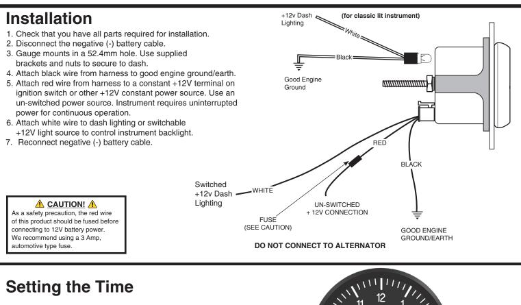
Use the two buttons on the face of the gauge to set the time. The left button moves the hands counter clockwise. The right button moves the hands clockwise.
