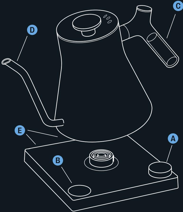
**A DIAL** One quick press to turn the kettle on or off. One long press to start the Brew Stopwatch. Turn to select the temperature.
