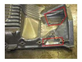
After these modifications are done you can fit the JSP engine mount brackets to the engine using the supplied m10 hardware. You will use the AE86 rubber engine mounts on these brackets to mount the engine to the crossmember.
