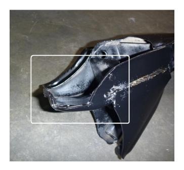
The oilpan needs to have a section removed and patched as well as a lower edge shaved off. The area in the middle lower portion removed is needed for cars still using a power steering rack. If a manual steering rack (recommended) is used it is not required to modify this area.
