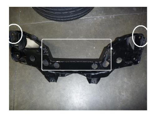
Notice the highlighted areas of the middle and corners as the areas of the crossmember that need to be modified. The middle is to clear the oil pan, the outsides are the clear the swaybar.
