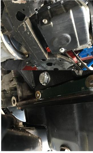
After these modifications are done you can fit the JSP engine mount brackets to the engine using the supplied m10 and m12 hardware.
