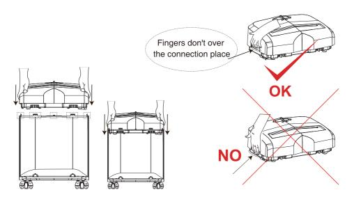
① .Install shredder's head: Take the shredder's head to aim at shredder's body and press down after the shredder's head aimed at shredder's body(Please don't overexert and damage the shredder's body.)
