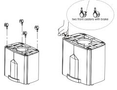
④.Install shredder's casters: Tip over the shredder's body with basket on a flat and stable surface place, casters aim at caster holes and press down (Two front casters face handle direction).
