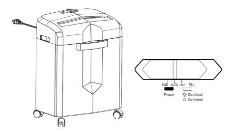
(9).Plug in and move the "control panel" to Auto , power light is in blue(finish the Installation ) .
