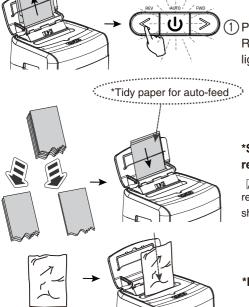
Pull out the jammed papers and press the REV button.( Auto button in red and blue light with flashing)
