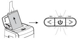
Auto button is under red and blue light with flashing or red with flashing, It means the "Auto-feed opening(red and blue light with flashing)" or Manual-Feed Opening(red with flashing) is over its capacities, need to take out the excess papers.
