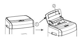
1.Open the Auto-feed Supporting plate and the Auto-feed fixed rod to make the Auto-feed Connecting plate(top and bottom) straight. (when open the Auto-feed Connecting plate under straight status, there will be a voice like a click)
