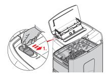
(3) Move the Auto-feed cleaning button and make the paper scraps into the basket.
