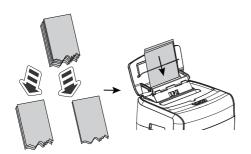
\*Suggest to separate the jam paper to re-feed shredding in manual-feed.
