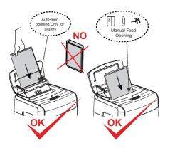
4.Feed the tidy papers to "Auto-feed opening" or feed the papers to "Manual Feed Opening".(Auto-feed opening:Max 110 sheets Manual Feed Opening:Max 12 sheets)
