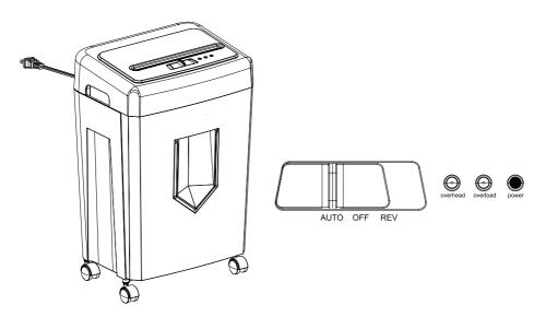
8.Plug in and move the "control panel" to Auto, power light is in red (finish the Installation).
