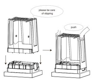
⑤.Install the trash can: align the body of the shredder with the body of the shredder, and then press down after the body of the shredder is aligned with the head of the shredder (please do not use too much force to avoid damaging the body of the shredder or the head of the shredder).
