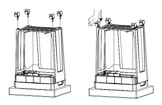
⑥.Install shredder's casters: Tip over the shredder's body with basket on a flat and stable surface place, casters aim at caster holes and press down.
