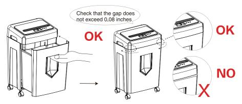
⑦.Put the basket of the shredder on the body of the shredder to close it, and then check whether it is well installed around the shredder, and the clearance between the nose and the body is no more than 0.08 inches.
