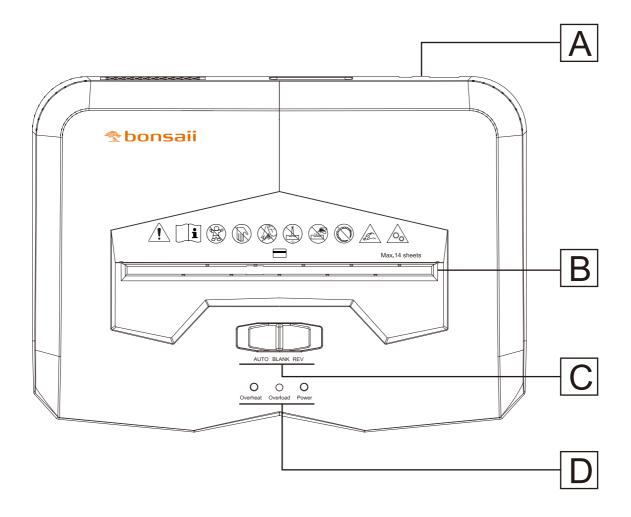
A: Main Switch - ON / OFF B: Feed Slot
