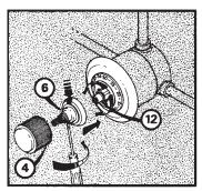
Let the water flow and bring this to a mean temperature by actuating the bushing (12). Note this temperature. Place the pointer assembly (6) on the bushing and position the "red" index opposite the graduation corresponding to the temperature noted.
