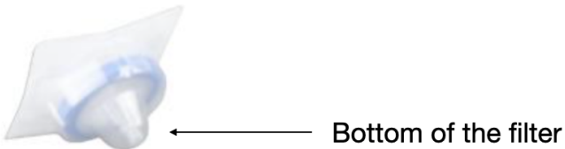
Figure 1. Filter. Avoid touching the bottom of the filter once it's out of the package. Hold the filter by the colour ring.
