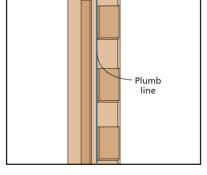
3. If installing new jambs, measure down from the underside of the top of the jamb 7" to position the top of the top hinge. Measure up from the bottom of the slab 10" to
