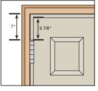
position the bottom of the bottom hinge. Place the middle hinge halfway in between.
