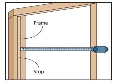
(usually 1/4"-1/2" taller) to allow 1/8" clearance on the head jamb and allow the slab to operate without rubbing on any flooring.
