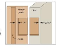
6. Using a template, mark the jambs and slab where the hinges will be mounted. Using a
