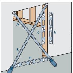
• The face of the rough opening must be in a single plane (E) with less than 1/8" twist from corner to corner. • Do not install the slab unless the jamb meets the above conditions. Professional assistance may be necessary to correct any problems before installation.
