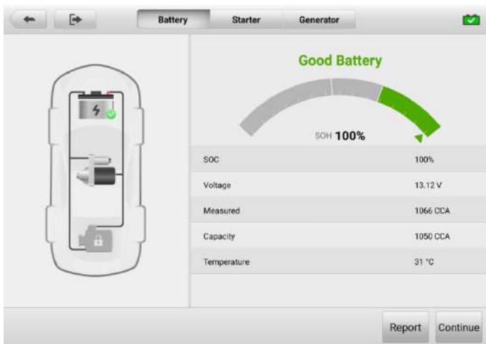
Figure 20-6 Battery Test Results Screen
