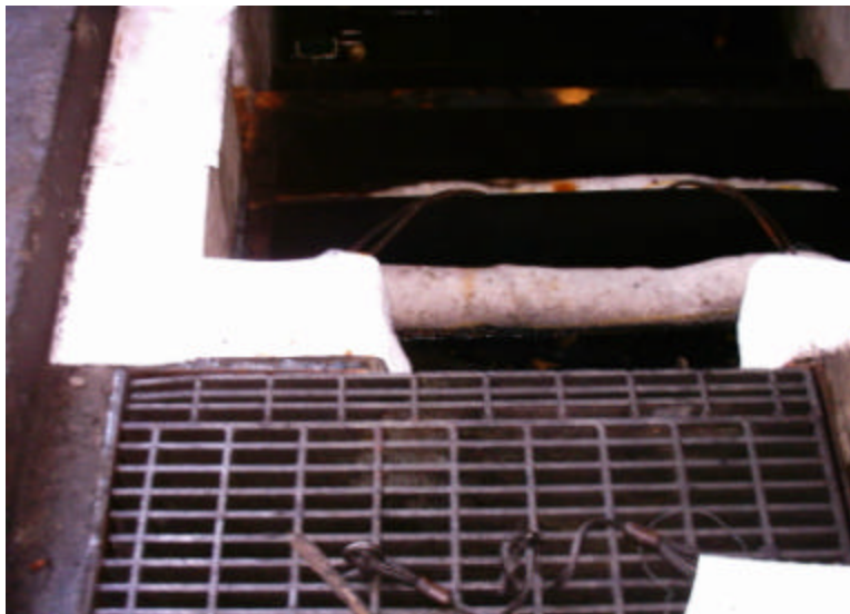
Figure 3. Showing the metal trough and the walls of the channel covered by residual oil released during washing. Cleaning of the trough and channel requires 2 days of operating time.
