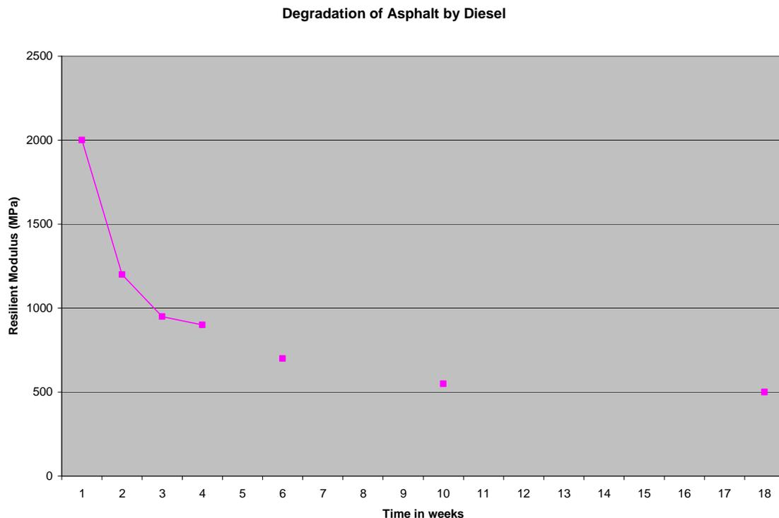
**Figure 7. Laboratory analysis of effect of diesel on core samples treated with diesel simulating road conditions.**
