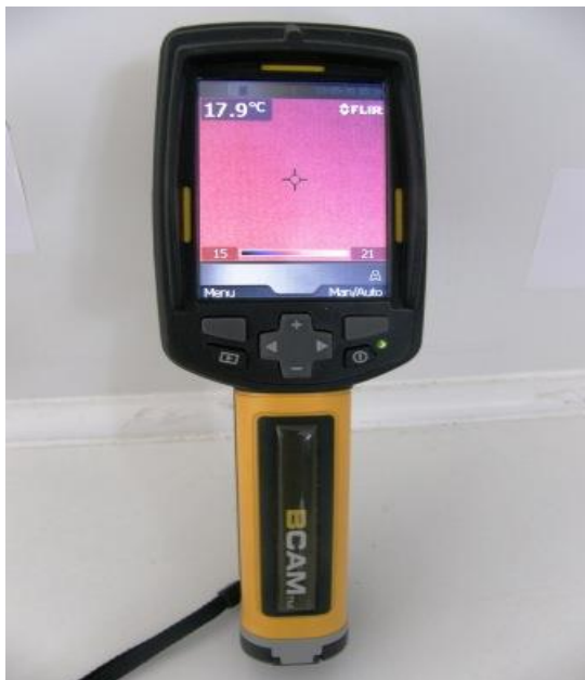
Thermal imaging camera for detecting Underground heating pipes.
