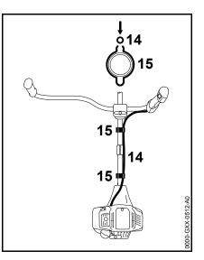
• Push the throttle cable (14) into the retainers (15).
