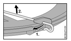
Disconnect wire rod from the transport guard.
