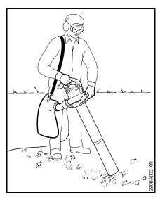
Your vacuum shredder is designed for two-handed operation. Hold and operate the power tool with your right hand on the control handle and your left hand on the assist handle (union nut). Wear the catcher bag shoulder strap over your right shoulder, not across your chest. This enables you to quickly remove the power tool and catcher bag in an emergency.
